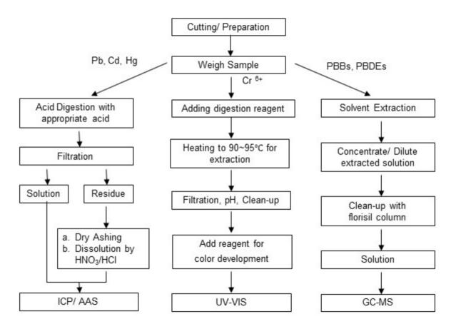
Note : 1) Boiling water test method was also performed for Cr (VI) analysis in metal sample.
